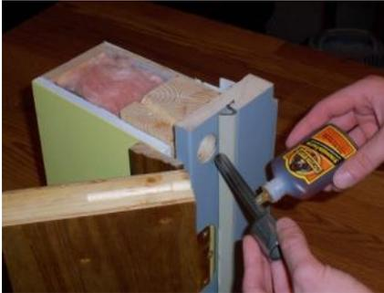
9 Apply appropriate glue to Detail #1 and install into doorframe. Rotate Detail to align with hole properly.
