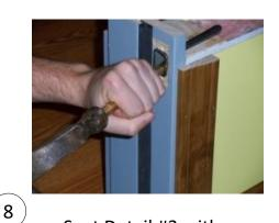
Seat Detail #3 with a hammer and punch to move past the designed interference.
